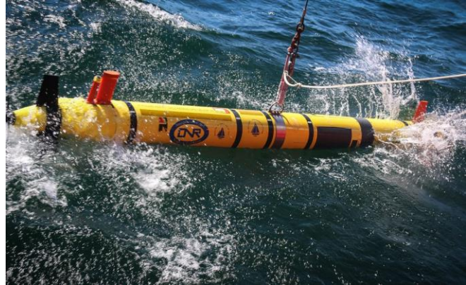
Figure 1. A U.S. REMUS 600 multi-use UUV deploys during BALTOPS 2018. 13
