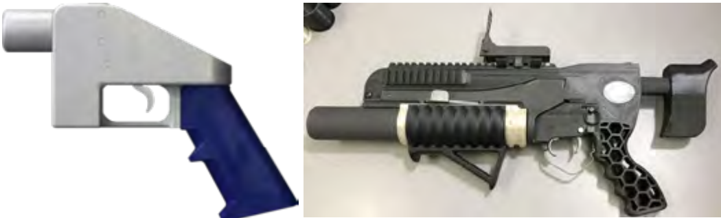
Figure 1. Comparison of the first 3D-printed gun (the Liberator, stereolithography [STL] geometry files were released to the public in 2013), left, and a US Army Armament Research, Development, and Engineering Center (ARDEC) 3D-printed grenade launcher (RAMBO) in 2017, right.
