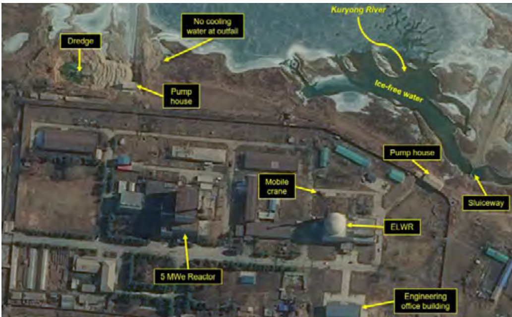
Figure 1. Commercial image and annotation appearing on the 38North website and used to monitor activity at North Korean nuclear facilities.
