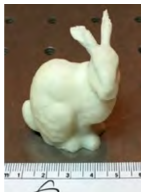
Figure 12. An example of using open-access print files in energetic printing. The Stanford Bunny produced from an FDM-based explosive material. 23
