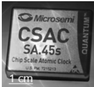
Figure 9. Space-rated rad-hard chip-scale atomic clock. 34
