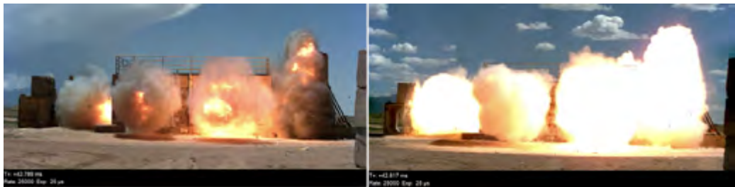
Figure 9. Testing of reactive cases: Baseline in steel case (left) and LANL Al-Foil reactive case (right).
